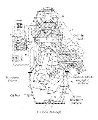
The Examiner identifies the above as "Annotated Figure 1 of Elsbett with the modular combination of Sachdev." Ans. 4. The Examiner applied a pair of dark marks labeling them "Cylinder block engaging surface," which identifies the interface between the upper "Cylinder head" and an intermediate "Structural Frame." This is distinct from the Examiner's identification of the "Oil Pan Engaging surface" which is the interface between the intermediate "Structural Frame" and the lower "Oil Pan."
